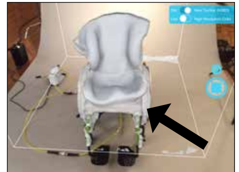
Make sure the colored foam layer of shape capture base is scanned.
