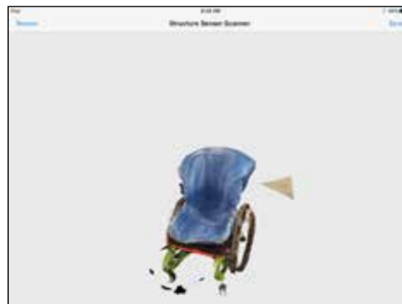
Finished processing, spin image on touch screen to view all sides of scan and ensure trim lines are visible.
