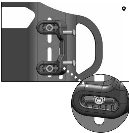
4. Wheelchair frame widths can vary from chair to chair. If you have any trouble aligning the mounting brackets with the attachment pins, you can easily adjust the width of the Java Back to fit perfectly.
