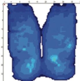
Performance on the Ride Forward Cushion is consistent at room temperature, and as it warms over the same 30 minutes. It is the contour of the Ride Forward Cushion that protects bony prominences. The visco-elastic material is in place for comfort at the proximal thighs and posterior-lateral buttocks where Ride purposely elevates the forces of support.
