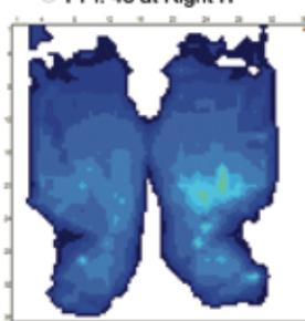
The cushions were then frozen to a temperature of 23 degrees F. The competitor cushion is hard and is not safe to sit on. The Ride Forward demonstrates improved off-loading of bony prominences when stiffened by freezing. The Ride Forward is safe to sit on at virtually any reasonable temperature, even frozen.
