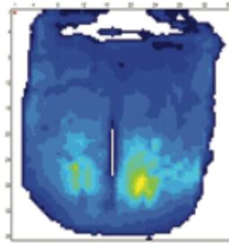
After sitting for only 30 minutes, the competitor cushion's visco-elastic material displaces, causing the sitter to bottom out on the polyurethane foam base. This creates a potentially dangerous situation.
