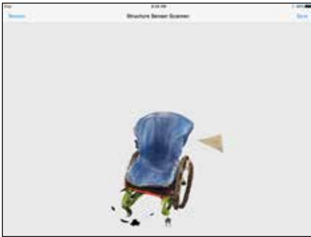
Finished processing, spin image on touch screen to view all sides of scan and ensure trim lines are visible.
