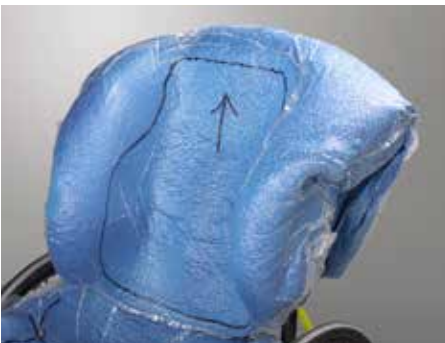
Trim lines marked.
