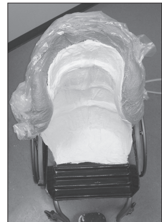
Properly finished cast with plaster extended into bottom of simulator pan with the blue foam removed. Replace blue foam in pan for shipping after removal of cast.
